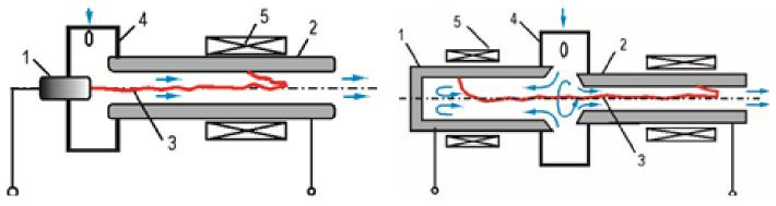
Fig. 2. Schematic diagram of single-phase plasma torches with gas stabilisation and the self-adjusting arc length: a) with the internal pin electrode and b) with two tubular electrodes (1-cathode, 2 – anode, 3 – electric arc, 4 – swirl chamber and 5 – magnetic coil) [12]
