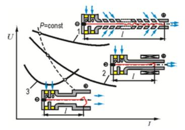
Fig. 1. Current-voltage characteristics of arc in the three types of linear plasma torches [1, 5]: 1 – plasma torch with the inter-electrode insert, 2 – plasma torch with the self-adjusting arc length and 3 – plasma torch with the edge in the electrode extension area
