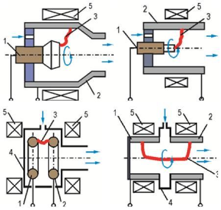
Fig. 3. Schematic diagrams of plasma torches with magnetic discharge stabilisation: a) coaxial system with the cold internal electrode, b) with the hot internal electrode, c) with cold ring electrodes and d) with cold tubular electrodes (1-cathode, 2 – anode, 3 – electric arc, 4 – swirl chamber and 5 – magnetic coil) [12]
